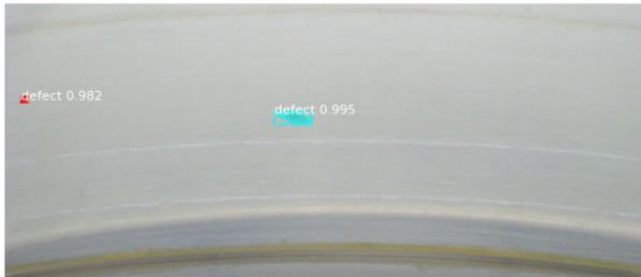
Fig. 9 Test Bearing Inference on Key Corrosion Locations
